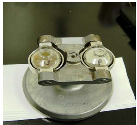
Samples of the wool washing effluent were analyzed via centrifuge to determine what type of machine would be needed to separate the solids, liquids and grease.
